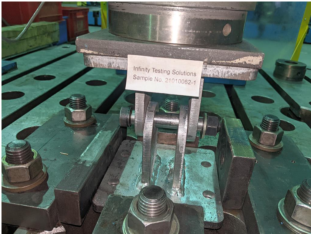
Figure 2: Sample during maximum load (43,000 lbf)
