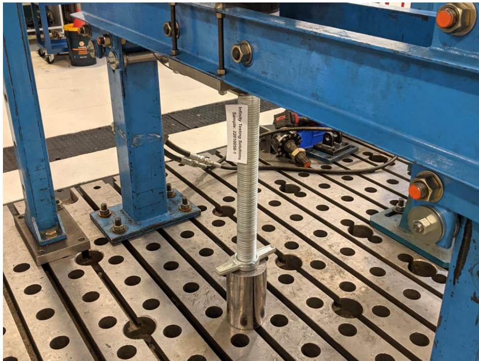
Figure 2: Clamp force test, hand tight + full turn, compressive load of 1,147 lbf
